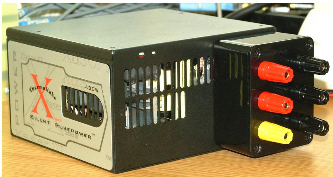
**Photo D.8:** *The main system power supply. This is a converted PC PSU, that provides a very high power source.*
