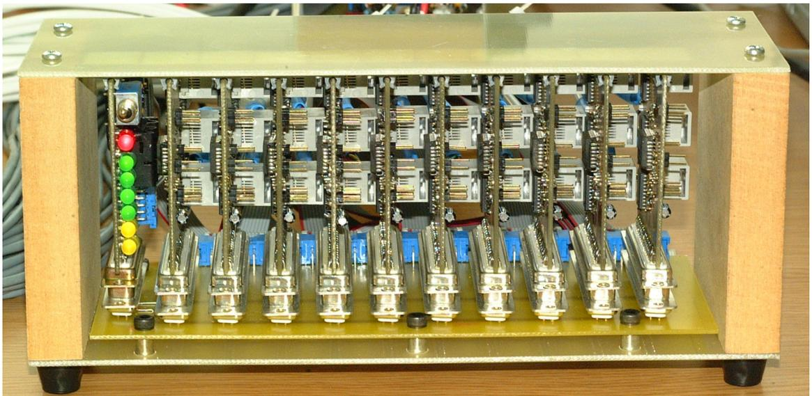
**Photo D.10:** *The front view of the monitor and programming data channelling boards. The column of LEDs to the left show which bioNode is currently selected for programming.*
