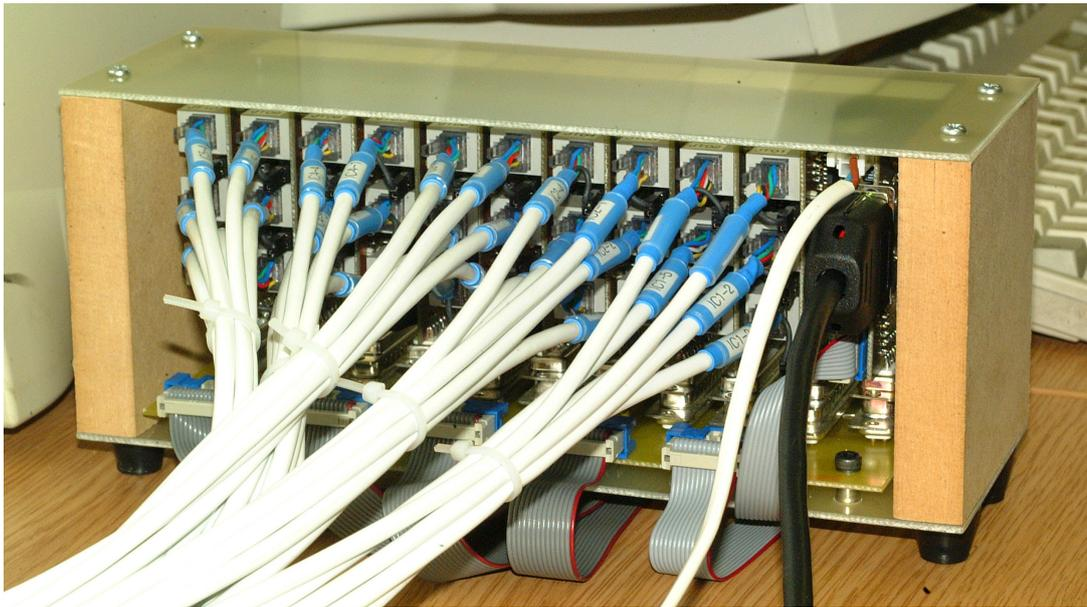
**Photo D.9:** *The thirty bioNode data umbilicals connect to a bank of boards that channel monitoring and programming to and from the main supporting PC.*
