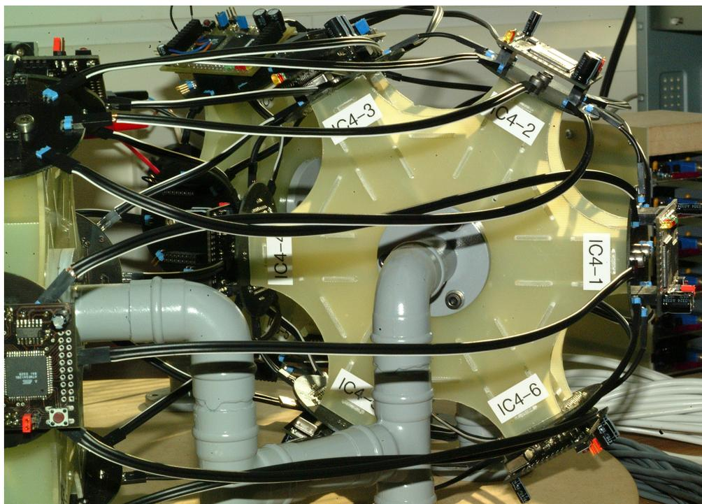
*Photo D.2: A close up of one of the platters that form the bioNode system's toroidal shape.*
