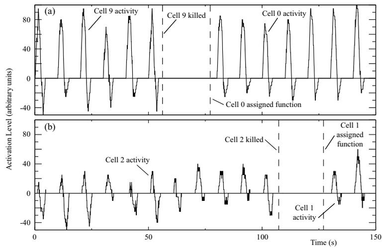
**Fig. 9.** Graph of activity levels in four different cells as they become activated and deactivated, demonstrating the systems ability to deal with microcell loss.
