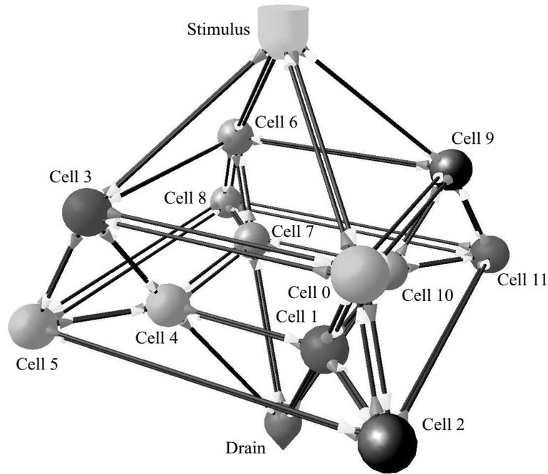
**Fig. 6.** A representation of the multiprocessor system. Cells 0, 4 & 5 and Cells 1, 3 & 11 perform different processing tasks. Cells 2 and 9 have been killed off to demonstrate fault tolerance. The remaining cells are redundant. The main system input (Stimulator) and output (Drain) are also shown.
